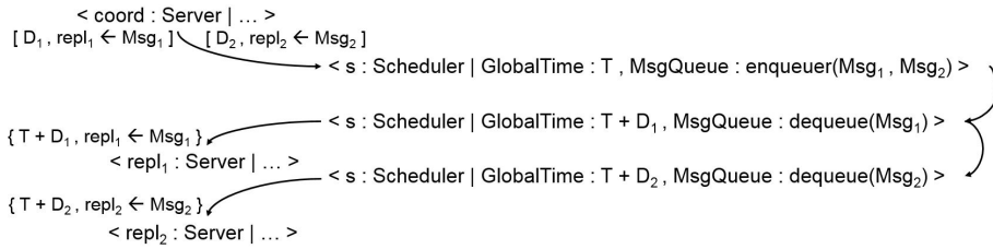
Fig. 2. Visualization of rewrite rules for forwarding requests from a coordinator to the replicas
